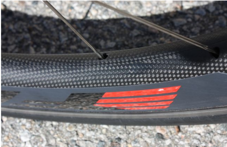
A proprietary aluminum rim, designed by FLO, is co-molded to a 3K carbon fiber fairing that's also a FLO proprietary design. The wheels are manufactured in Taiwan.
